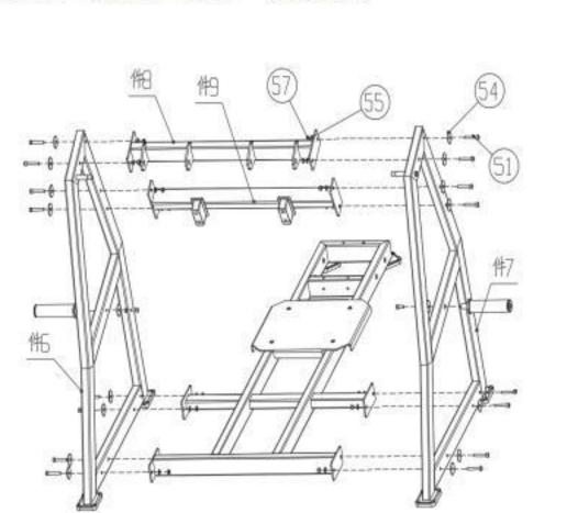
Step 2: Join # 2, # 3, # 4, # 5, and # semi-finished product 1 to form # semi-finished product 2 using the following method:
